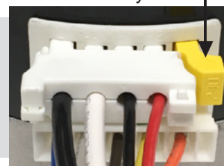
Yellow Voltage Plug 230vac Systems
